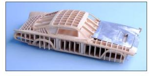
The Bertone Carrozzeria used a time-tested approach to building the second *Lynx* prototype. Using the first *Lynx* prototype that was shipped to Bertone for reference, the craftsmen built a wood buck over which aluminum sheet metal was hand hammered. As each panel was completed, it was removed and heli-arced to the Bertone-built metal framework of the 1:1 car. **This wood buck, and workbench - built by Jim Fernandez to match vintage photographs - exhibits how wood was used to establish**
