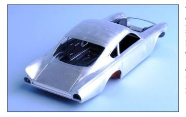
This model *of Lynx-3* depicts the aluminum body during its construction phase at Bertone, where *Lynx* prototypes 2, 3 and Mill's personal *Lynx* coupe were built. **Andy Kellock replicated the handhammered aluminum body for Lynx-3 that craftsmen at Bertone Carrozzeria crafted for Lincoln-Mercury chief Ben D. Mills. Mechanical details will be added by Mark S. Gustavson with the completed model placed in the replicated Bertone body assembly jig created by Jim Fernandez.**
