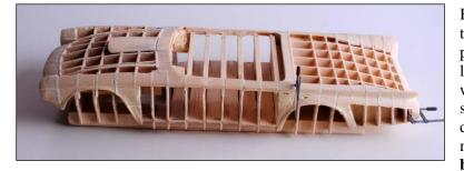
Bertone also built a wood buck over which the exterior metal shapes for this *Lynx* prototype were hammered. Forming the large flat rear deck of the *Lynx* convertible was more difficult than the more complex shapes of the hardtops because it was difficult to prevent "oil-caning" when mounted to the body. **This wood buck was built by Jim Fernandez.**
