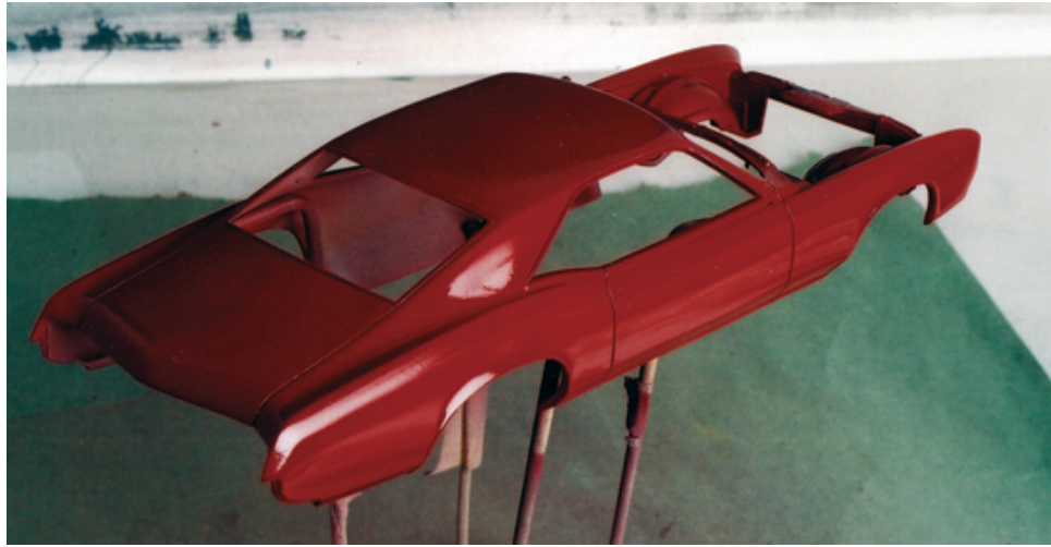
Figure 11.17: Thin out the color by 10 percent and lay down two more color coats. At this point, the paint on your model should look like this, but lacquer will “pucker” up a bit as it dries, necessitating polishing.
