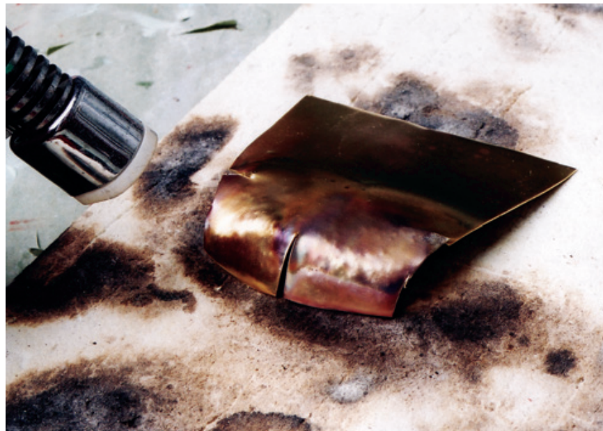
Figure 10.47: Before we solder the panel, we need to anneal the sheet brass. As you shape the panel by tapping on it, you are work-hardening the material and we need to reverse that process. You need to lightly play a flame across the panel once it has been placed on a fireproof material like this thermal panel—don't do this near any flammable material! You should not heat the panel to the point where it sags, just get it obviously hot and then let it cool down without quenching it in oil or water.
