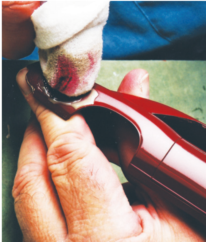
Figure 11.25: When you need to rub out paint around a wheelwell, rub the polish into the surface and then rotate your shrouded finger up and around the sharp crease. Note that this surface has not been sanded—even with 2000-grit paper—because of the care taken in the application stage, which consisted of the application of the last three coats of color over a carefully-sanded finish. Note the very slight orange peel just forward of the wheelwell, midway up the panel.
