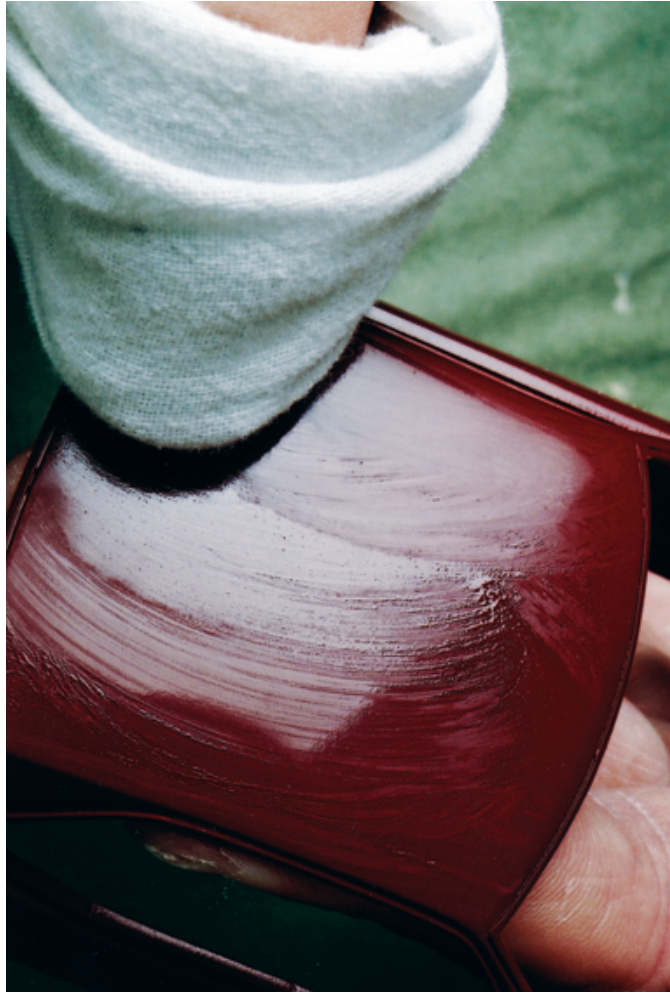
Figure 11.22: Gently rub the polish into the surface, using a roughly circular motion. Any particular area may take four to six minutes to produce a mirror shine. Go gentle on the pressure, and always support the panel by placing your other hand underneath it. Watch to avoid rubbing too much on any sharp panel crease or other protrusion: You can rub right through the color to the sealer below.
