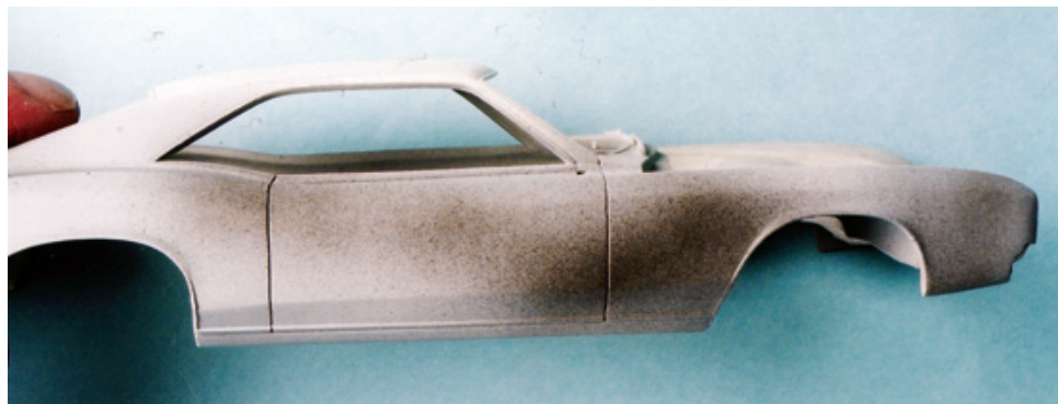
Figure 11.1: Once your basic bodywork is finished and primed, apply a light coat of very dark lacquer (preferably black) over the primed areas that cover your bodywork. The purpose of applying a guide coat is to detect high and low spots in your bodywork when the guide coat is sanded.
