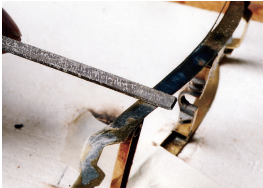
Figure 10.31: Using the same .100 by .020 strip brass, continue to add the top and bottom brass strips to the side frame rails, and then do the same on the underside of that side of the frame. Then repeat the boxing operation on the other frame rail. Since the frame is pinched in a couple of places, the strip brass can be bent (using a torch first to soften the metal) to fit, and then soldered.
