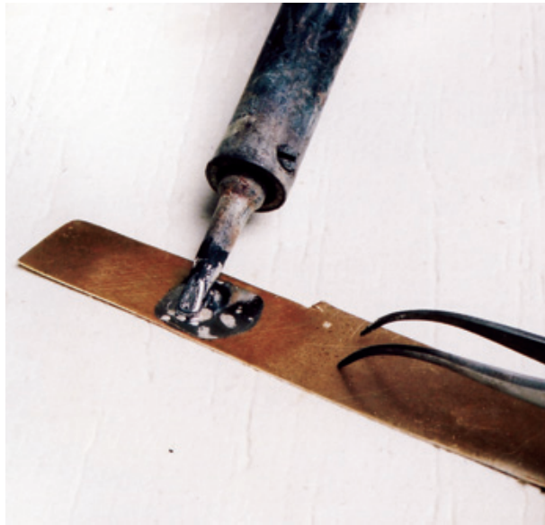
Figure 10.10: . . . in the deposition of the solder on the surface. Spread the solder around a bit, making sure that the solder flows out easily, and is shiny at the completion of this operation.
