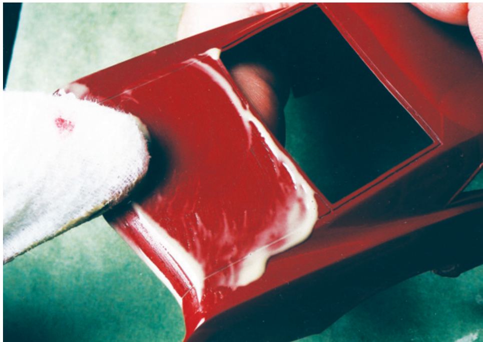
Figure 11.27: The trunk, as with other roughly square panels like the hood, can be rubbed out by consistently applying the polish in a circular pattern. You should also polish the trim around the “glass” so that, when you apply your Bare Metal Foil, the underlying surface is mirror smooth.
