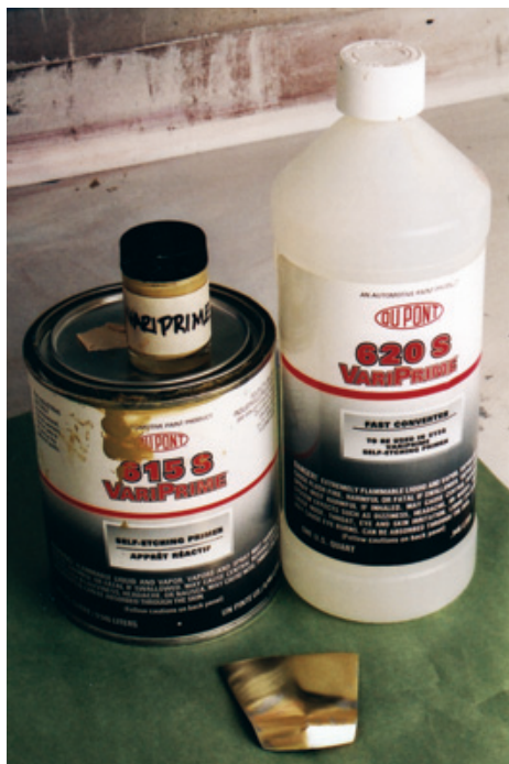
Figure 10.55: With the hood close to its finished shaped (it's shiny from being smoothed with a fine sanding stick), it's time to apply a good primer/sealer. Brass is an odd material, in a way, since it needs a coating that actually etches into the metal. I highly recommend Dupont's VariPrime because it "etches" the brass and can be applied directly over the filed brass panel. Mix the two parts 1:1. Be sure to use a dual filter respirator! Don't spray without such a mask. A regular dust mask does not work! Read the VariPrime Material Data Safety Sheet!
