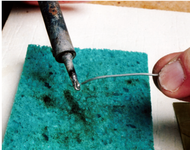
Figure 10.8: With the fluxed and completely heated soldering iron ready to go, press your silver-bearing solder to the tip and melt a bit onto the tip. You should melt only about 1/16" of a length of the solder.
