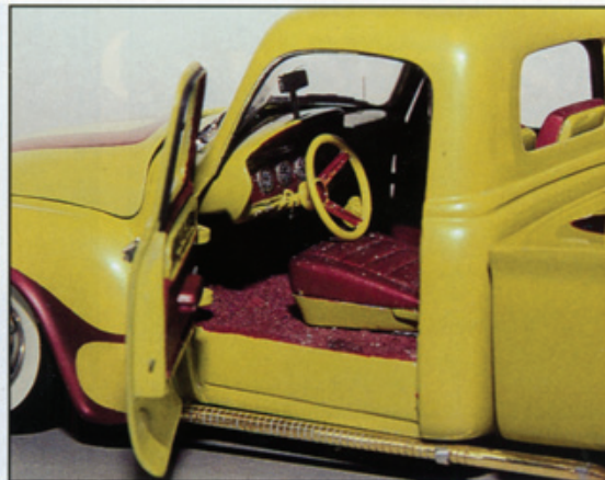
The interior components are painted to match the exterior. A low gloss clear has been applied over the 1962 Chevy bucket seats for a realistic vinyl look. The dash is poorly designed: The steering column is too low, dropping the small steering wheel almost to the seat. The gauge cluster needs to be raised to permit the steering column to be moved to a more realistic elevation.
