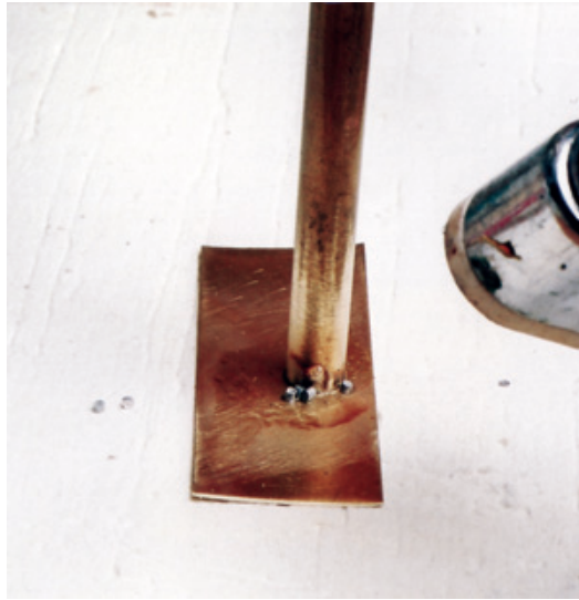
Figure 10.18: Play the torch flame onto the joint. Keep the flame low and move it around the perimeter evenly. Go slowly, and watch out for the heat!
