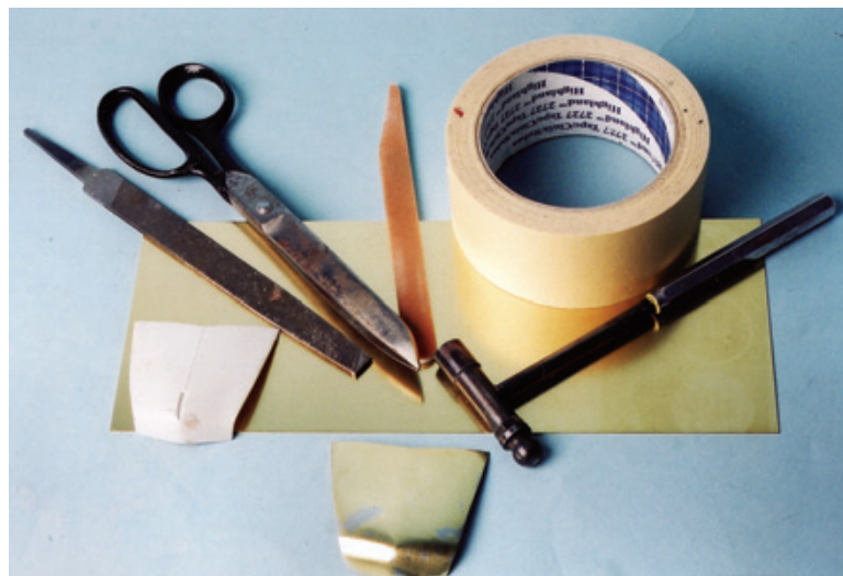
Figure 10.35: The equipment needed for forming your own brass panels is modest. A fine-tooth flat file, a pair of high carbon shears (available at any cutlery shop), a roll of tape, a hammer (from MicroMark), sanding sticks, and Evercoat catalyzed putty complete the items.
