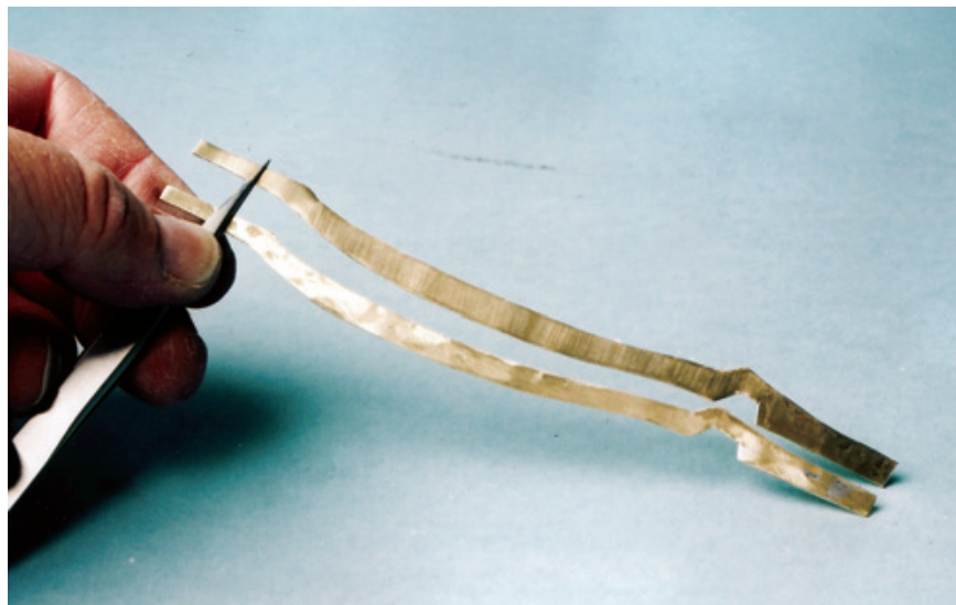
Figure 10.25: Even though there is a superficial resemblance between the two frame rails, the second one differs significantly from the first one. The critical part here is that both rails must match exactly. The way to reconcile the two parts is to spot solder them together.
