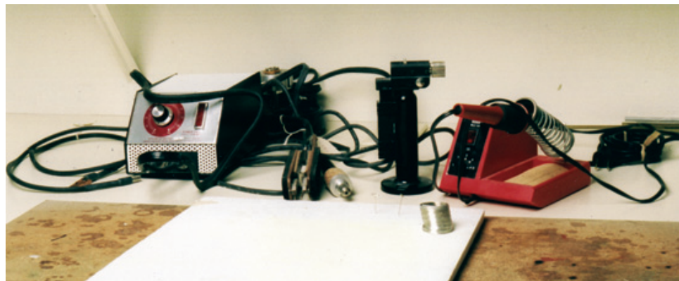
Figure 6.2: Set up your soldering workspace in a single work area and be certain to use a soldering base at all times. See Chapter 10 for soldering and fabricating techniques. (Mark Gustavson's shop/photo)
