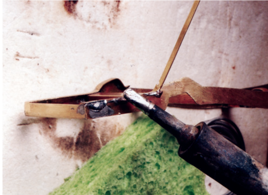
Figure 10.28: With the basic shape of the frame determined, it was time to add the top and bottom pieces to the frame rails. Lengths of .100 \times .020 brass strips were cut to length and soldered to the top and bottom of the frame rails. If a more precise jeweler's torch had been available, it would have been used with plenty of heat sinks. The problem with not having the solder hot enough is seen here at the back of the frame rail—too much cold solder has clumped up. I fixed it by clamping a heat sink at the point where the two most rearward frame cross-members met the frame rail and “pulled” molten solder until the solder ran the length of the strip brass.
