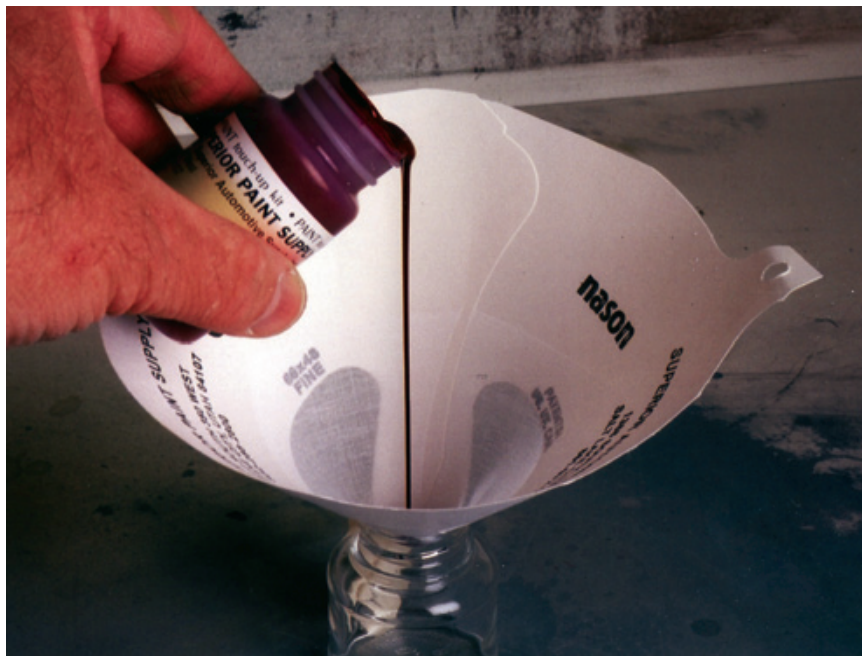
Figure 11.11: As the primer cures, it is time to mix up the top coat. In this case, we're using a 1996 Hyundai color that is a rich wine red tone. Always strain the paint to remove debris. Pour the paint slowly and fill your bottle about 40% full, then add compatible thinner almost to the top of the bottle (leaving just a bit of space for proper agitating when shaking). Discard the strainer after each use. Dispose of all used thinner, lacquer-contaminated strainers and related materials in accordance with your local laws. Spray a test pattern to test for proper paint atomization. Remember, any mixing formula is just a guideline because the actual viscosity of each paint varies.
