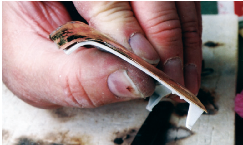
Figure 10.49: At this point, lay your hood on top of the original plastic panel. Note how the soldered area has buckled upward a bit. Gently tapping down on the outside of the part and then tapping up on the lower area will correct this minor difficulty. You'll encounter this sort of problem often, but it's easy to fix.
