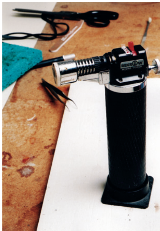
Figure 10.15: A butane-fueled torch is a handy investment. This setup works reasonably well: Get a unit with a base to keep it from tipping over. Its only drawback is that the flame is a bit too large for really fine work. A proper jeweler's torch would be better for the additional reason that the "pressure" of the flame won't move solder around.
