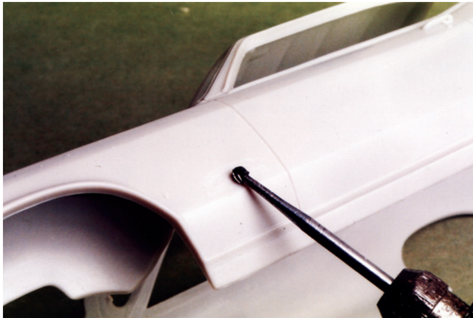
Figure 9.7: To remove molded-on emblems and chrome trim, use a rotary power tool with a round cutter and lightly excavate the surface. Wash the body thoroughly in a good-quality liquid dishwashing soap that does not contain silicone, and use an old soft toothbrush to lightly scrub the surface and all recesses.
