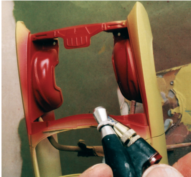
Figure 11.12: After blowing out the door reveals and other lines (away from your painting area), again gently wipe down the surface with the tack rag. Start by applying your color directly onto the sealer (our color is a “high-solid” and covers quickly). Your airbrush needs to be about 6–8 inches away from the surface and moved with moderate speed (use a test body to determine the best technique for each color). On this job, I used a Badger 350 with a fresh coarse nozzle and tip and the color was shot between 35–40 psi. Your first applications of color should be in recessed areas.
