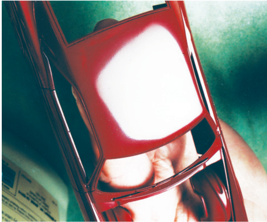
Figure 11.19: Here's the roof after the lacquer color coats have dried for about 10 days. Note that there is a slight puckering on the surface (commonly called orange peel), and this is perfectly normal. Our chosen polish will smooth out this surface to mirror smoothness. Do not sand this surface at this point.
