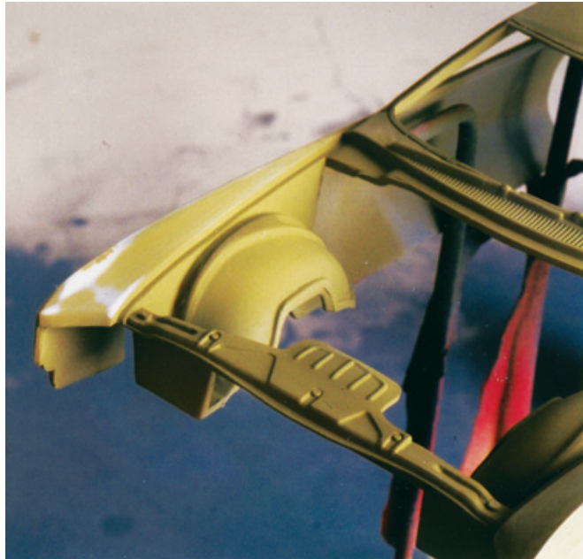
Figure 11.8: You may find that some surface flaws persist even though you were careful. In this case, a slight problem was missed on the left front fender. Once the sealer had thoroughly cured (about an hour), a fine-grit sanding stick, with water, was used to sand the offending area. After the model was washed again and dried, just this small area was re-sealed. You can apply the sealer directly over bare plastic.
