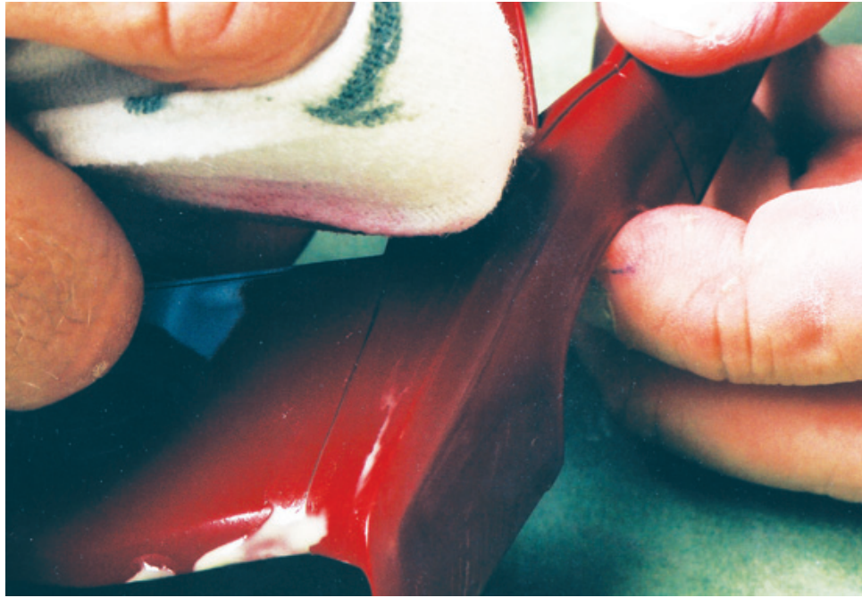
Figure 11.24: The same process is used on the top of the fender. By placing your index finger inside the soft rag which is lightly soaked with either M-3 or Finesse-It, you can get a mirror finish along a recessed area like this one. Watch the progress of your work to avoid rubbing through on a sharp panel crease.
