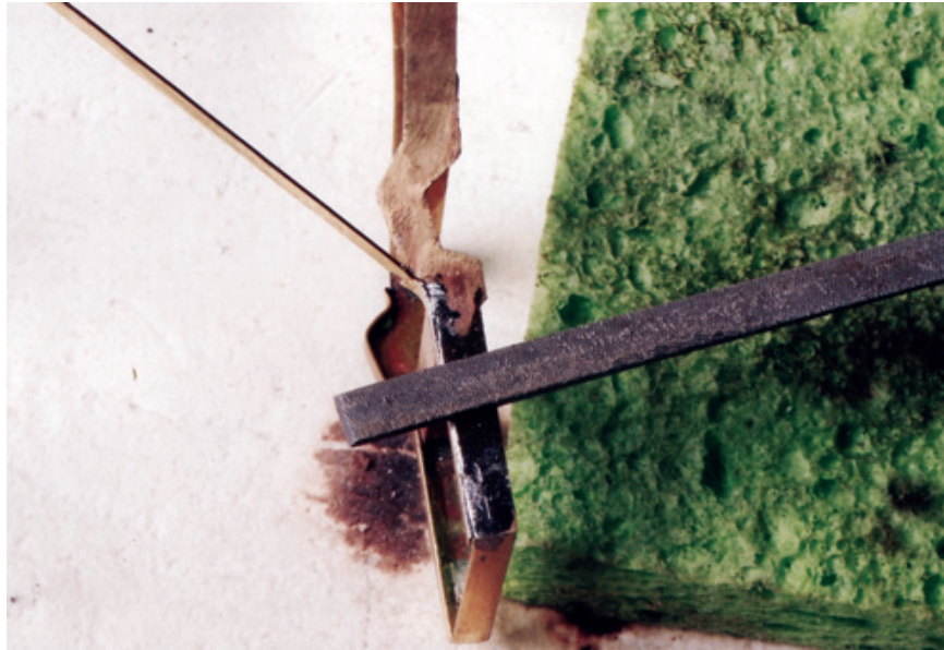
Figure 10.29: After a few quick passes with a flat hobby file, check out the neat and authentic look of this partial boxed short length of the frame.
