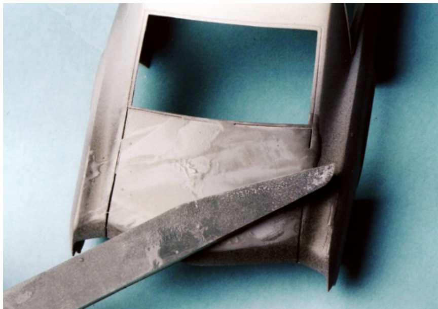
Figure 11.3: You should wet sand the guide-coated surfaces, using a medium sanding stick to prevent surface irregularities that might be created if you "finger sand." Sand at an angle to the panel rather than parallel to the panel's shape. Note the sanding sludge created here; just be sure to wash it all off periodically.
