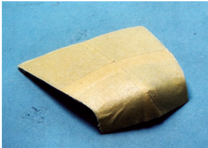
Figure 10.38: Carefully trim the tape to the perimeter of your part with a fresh hobby knife blade. Your part should look like this now.
