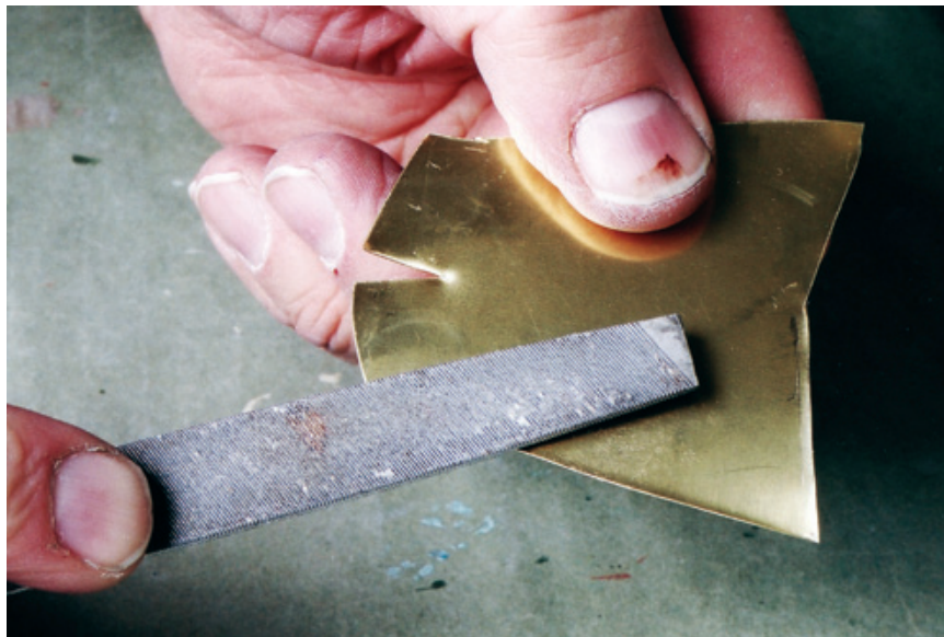
Figure 10.43: Use a fine-tooth flat file to file down the raised edges around the perimeter of the part. This will also reduce the chance of cutting your hands—remember this is metal and it can be sharp!
