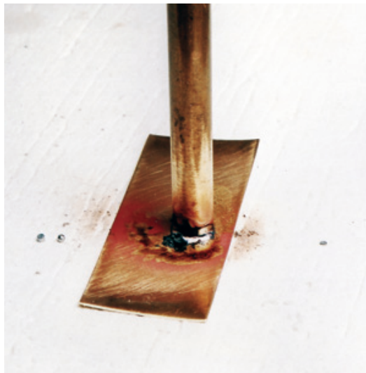
Figure 10.21: Continue to heat the interface between the two parts so that all of the solder balls melt and flow around the circumference of the tubing. Now, can you think of parts that can be made this way? Think about all the ways you can use soldering your next project.
