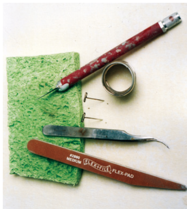
Figure 10.3: You'll need a few more tools, too. A medium-grit sanding stick is used to clean the metal surfaces. Tweezers are used to place small balls of solder, and can also be used as a heat sink, which is necessary to thermally “insulate” prior work from the heat used in subsequent operations. The hobby knife is useful to cut solder. Small brass pins can help to locate an assembly of parts to
