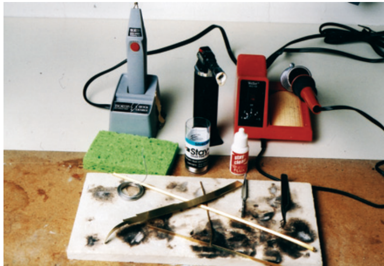
Figure 10.1: An adjustable-temperature soldering iron, with a safety holder, is best. Weller makes a good unit; this was purchased from MicroMark. The torch uses Butane and should always be filled outside to assure plenty of ventilation. This unit has a trigger to ignite the gas, and the flame width is adjusted by moving the red slide valve mounted on top of the torch.
