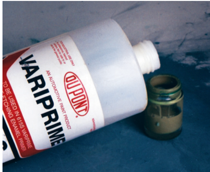
Figure 11.6: Blow out the panel lines with your airbrush—running just air, of course—and then set the model aside. Now it’s time to mix up your sealer, Dupont’s VariPrime mixed 50-50 with the Activator. No further thinner is necessary. Shake the airbrush bottle for a few minutes to assure a good mix. The VariPrime mix has a pot life of about 48 hours, but always re-shake the bottle before each use.
