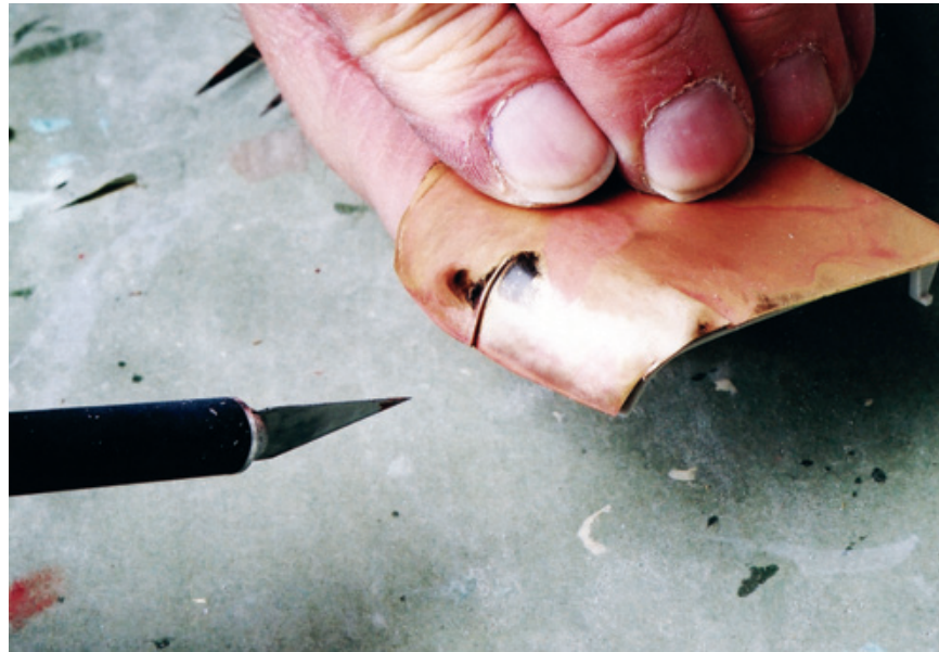
Figure 10.46: Relief cuts need to be made on both sides of the hood, as shown. The vertical line at the front of the hood is the cut made initially in the tape pattern—note how shaping the panel has closed the gap. The uneven bottom edge on the front of the hood is not a problem—this is the natural result of the hammering process. We'll trim it later.
