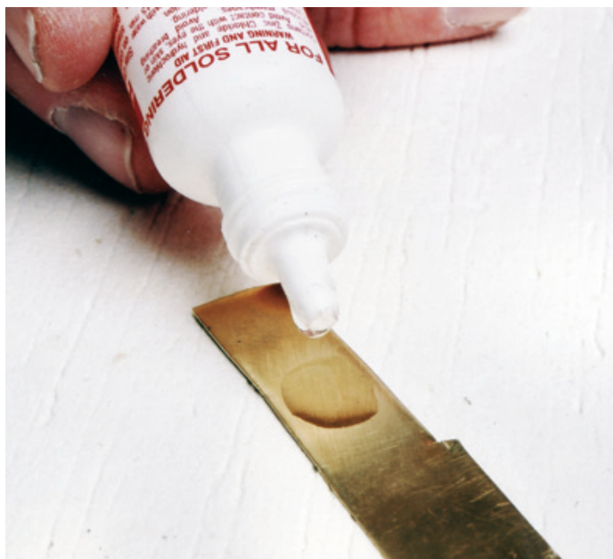
Figure 10.7: Apply a bit of flux to the two surfaces to be joined together. Rather than squeezing out a puddle of flux (as here), it would be best to use a glass eyedropper to avoid flooding the surface. Stay Clean-brand flux is an excellent product.
