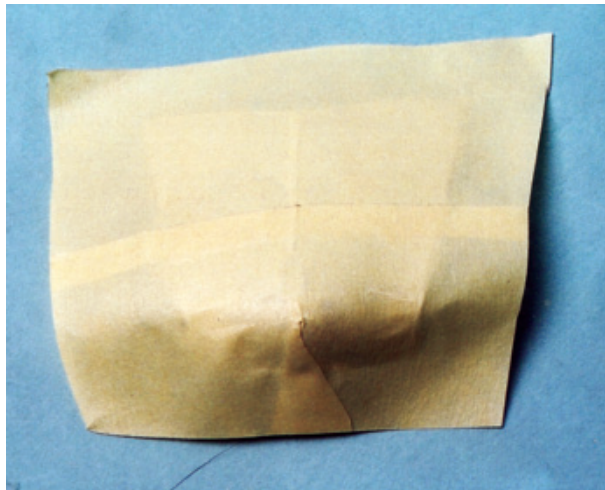
Figure 10.37: The first step is to use a roll of 4" masking tape. We need to make a pattern, so cover the hood with tape, using only two pieces laid out lengthwise. Try to pull the tape tight over the curved corners, but don't worry if the tape bunches up as it has here at the front of the hood.
