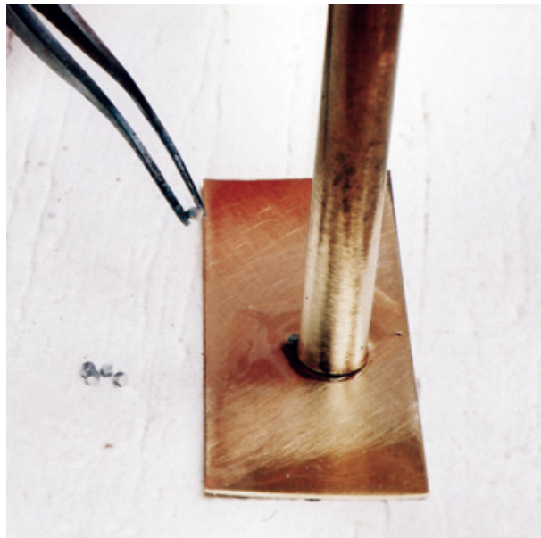
Figure 10.17: Lightly sand and flux both surfaces. After fluxing both parts, place the second piece atop the first, and then carefully place the small soldering balls equa-distant around the perimeter of the brass tubing to brass base interface.
