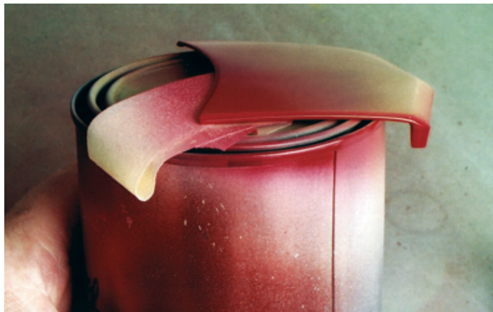
Figure 11.16: Go along the perimeter of the hood now, being sure to cover all of these vertical surfaces with a couple coats of color.
