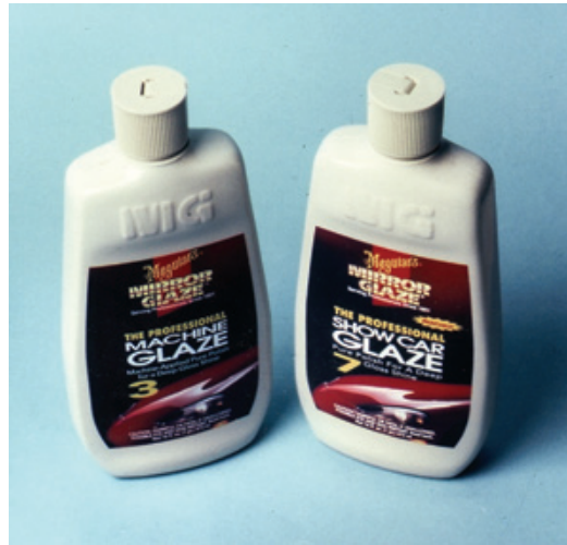
Figure 11.20: Now we're ready for polishing. You should visit your autobody jobber and acquire Meguiar's #3 and Meguiar's #7 paint polish or 3-M Finessee It! Don't ever use any silicone-based product—it will contaminate your work area (interfering with paint adhesion and preventing smooth paint application on other projects in the future), and will effectively prevent any paint repair to your model. Select genuine auto paint products and stick with them!
