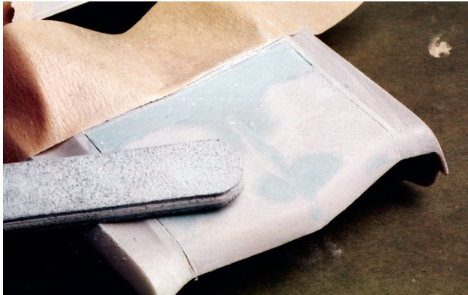
Figure 9.14: A similar approach is taken on the trunk. The peak was ground away and filled as in Figures 9.10 and 9.11; also, the vents were cut away and filled with a solid piece of strip styrene (you can't just fill in recesses—even with catalyzed putty—and expect to avoid “shadows” of those shapes later on). Here, the first coat of catalyzed putty has been applied, then rough-sanded to shape. More work will be necessary.
