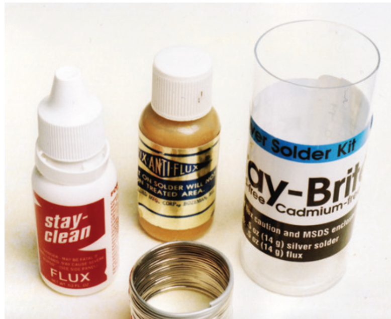
Figure 10.2: There are several types of solder. Make sure that you use a silver-bearing solder for strength. Don't use rosin core (electronic) solder or, worse yet, acid-core solder. For introductory uses, I recommend the Stay Brite kit that comes with liquid flux that can be squeezed from the flexible dispenser. Other types of solder are also available, including a paste format. You must use flux, regardless of the composition of the solder.
