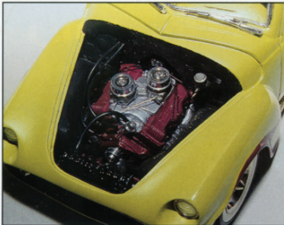
The AMT/Ertl 1962 Chevy 409 engine is a tight fit. The vastly narrowed engine compartment (reflecting the narrowed and tapered front fenders) just doesn't permit a big V-8 engine to be installed with normal operating items like an alternator in place. Additionally, you can't install the steering shaft! A long in-line motor needs to be installed. How about the inline GMC six cylinder from AMT's '51 Chevy Bel Air kit?
