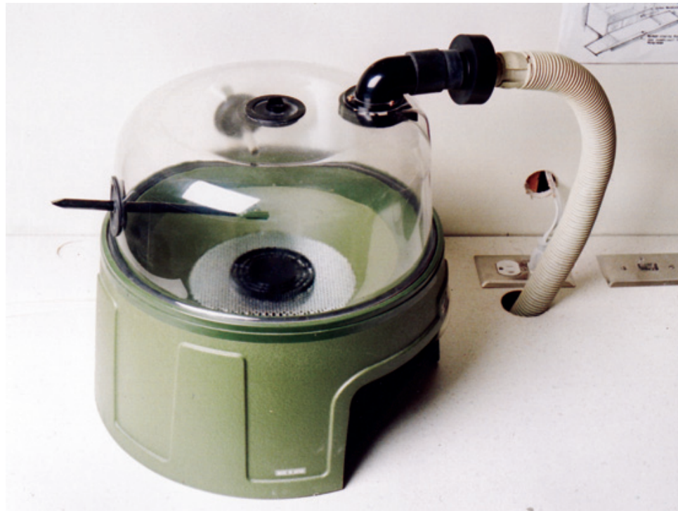
Figure 6.1: Media blasting is necessary to clean up a surface, or impart a texture, and can produce dust and particulate matter. Sequester such tasks away from your painting and final assembly area. (Mark Gustavson's shop/photo)
