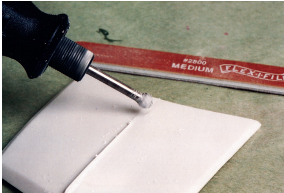
Figure 9.10: Sometimes, a panel is marred because the under-hood engraving appears in a “shadow” pattern on the outside. Though a real annoyance, it presents us with an excellent opportunity to discuss the techniques to correct this problem. In this case, we’ll also remove the over-scaled chrome molding on the hood. Grind out the shape, and then . . .
