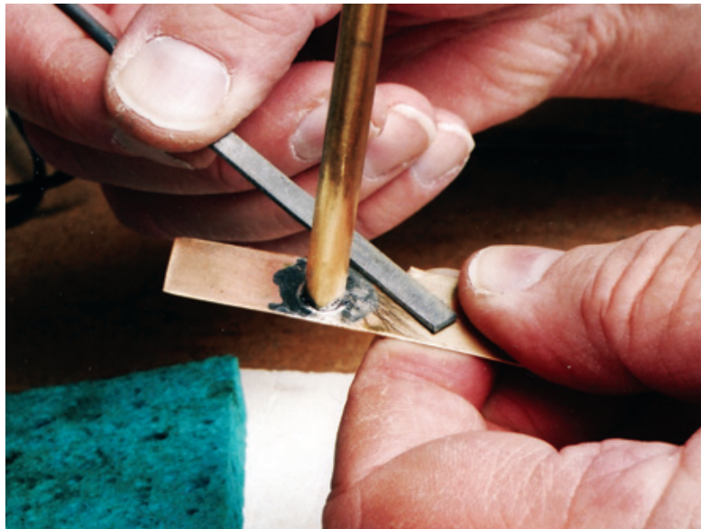
Figure 10.13: The mating surface can be cleaned up by using a flat hobby file. Be careful not to gouge the two brass surfaces. After the excess solder has been removed, use a medium sanding stick to remove any fine file marks.
