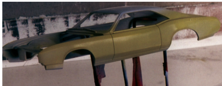
Figure 11.7: Once the lacquer primer has thoroughly dried, apply a light coat of VariPrime. Start on the underside of the fenders, then move to the recessed areas, and then move to the broad flat surfaces. Don’t be concerned if the sealer, when wet, appears to have a bit of an orange-peel surface; when curing, it flattens out considerably. In this photo, the roof has been left in primer to demonstrate the color difference. A uniform coat of the sealer should be allowed to cure for a few hours (the hood was also sealed at this time). Remember that the VariPrime actually “sets up” rather than dries since the Activator is a catalyst. This is a good time to remind you to be sure to use a two-cannister respirator: purchase a good one, use it, and keep it a sealed plastic container between uses. Replace the twin filters as recommended.
