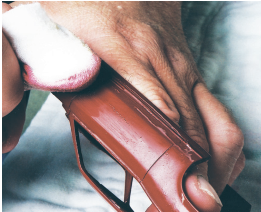
Figure 11.26: A long panel should first be rubbed with the polish along the length of the panel to cut down the orange peel. Once the finish is smooth—and don't be afraid to use the polish liberally—you should return to a series of small circular motions along the length of the panel.
