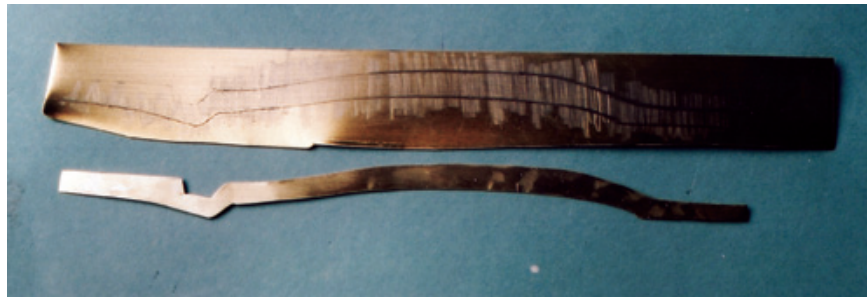
Figure 10.24: With the corrected brass master frame rail in hand, I traced it onto another piece of brass sheet and cut out a second frame rail.
