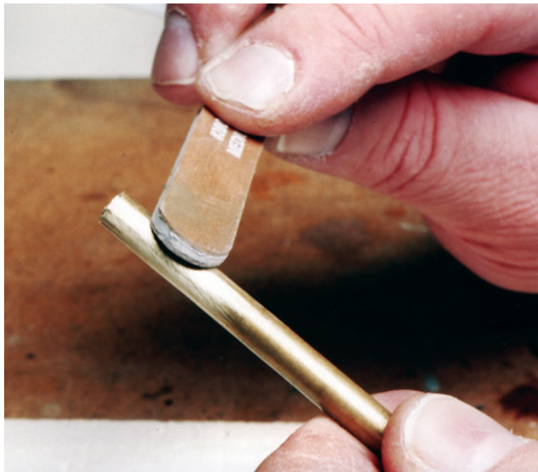
Figure 10.5: We'll be attaching a piece of tubing, so the base of the tubing is lightly sanded. Make sure that you clean up around the entire circumference of the part.
