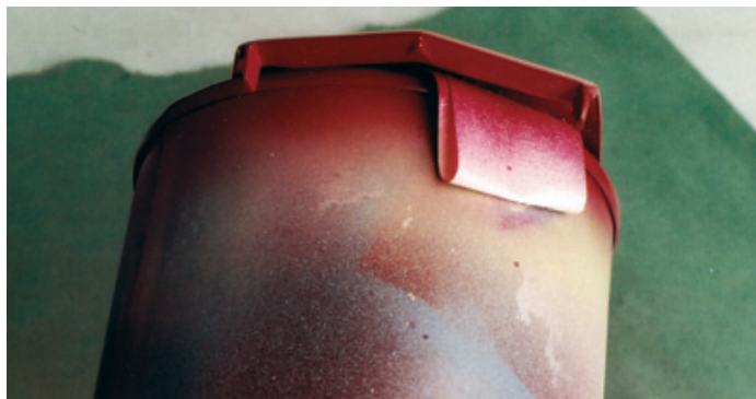
Figure 11.15: Paint your hood (and other removable panels) next by first painting the underside and the panel edges before proceeding to the top of the panel to avoid unnecessary overspray. Unless you're spraying a metallic or other custom finish (e.g., candies and pearls), the spray pattern is relatively unimportant.
