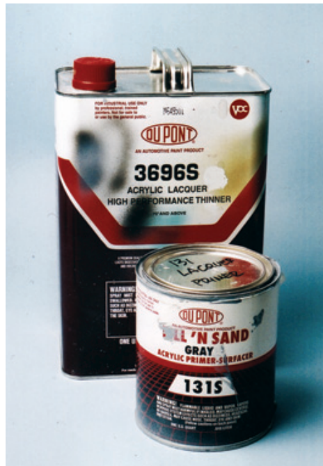
Figure 9.3: In the lacquer system, there are no better products than these. Never skimp by buying cheap thinner, and always mix the primer and thinner according to instructions. See Figure 9.4 for a mixing chart.
