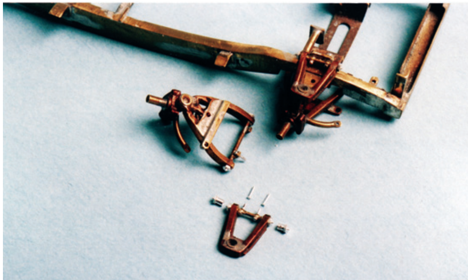
Figure 7.18: Cody Grayland machined the upper and lower control arms (complete with the bosses through which the mounting bolts are run) and the bolts that locate the control arm in the upper A-frame. The control arms are attached almost exactly as if they were 1:1 parts: the bushing slips over the shafts, which have been placed within the concentric “holes” through the pivot points in the upper and lower arms. The upper control arm bushing setup is comprised of five parts, as are the lower control arms.
