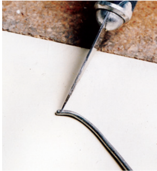
Figure 10.16: There is another, more delicate way to apply solder to the surface about to be heated: cut the silver solder into small bits with your hobby knife. Cut about 6–8 small soldering balls for the average soldered joint. This solder is being cut on the soldering surface because the textured surface keeps the small solder balls from rolling away.
