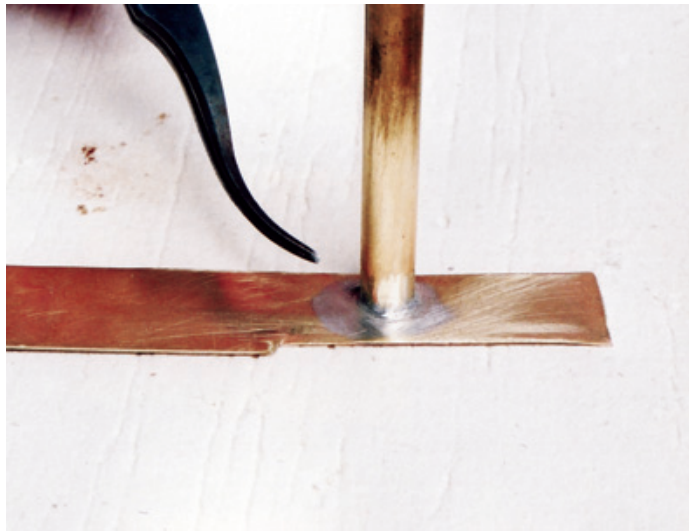
Figure 10.14: Careful work yields this tidy result. The surface can be further refined by using a fine sanding stick with water, followed by 1000-grit 3-M sandpaper. Before painting, it is recommended that you lightly scrub the soldered parts with a discarded toothbrush soaked in a 50-50 mixture of vinegar and water, and then rinse in plain water. This will remove any remaining flux that would interfere with paint adhesion. After rinsing and drying, you should use a professional etching primer like Dupont's VariPrime.
