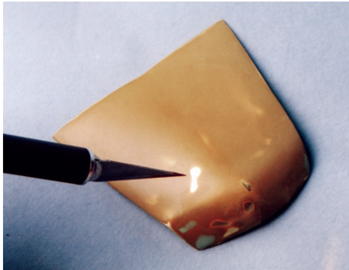
Figure 10.60: More sanding after the next coat of VariPrime will reveal still further slight surface irregularities, but things are getting better. Here the tip of the hobby knife points to a very slight high spot. Tap down that small area very gently. Note two small areas of sanded putty at the leading edge of the passenger side.
