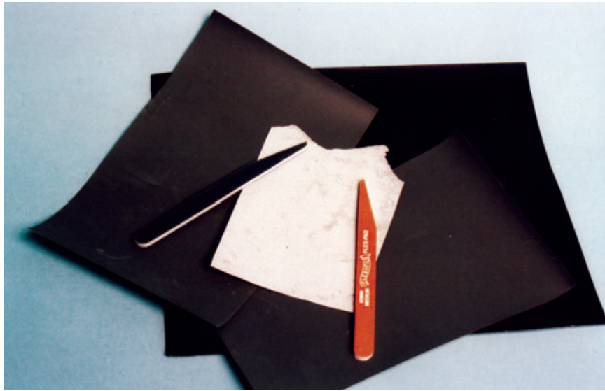
Figure 9.2: A great finish is no better than the surface preparation. You should acquire a range of the popular and ever-useful sanding sticks, some 150 dry autobody sandpaper (in the center), as well as some 3-M autobody 600 grit, 800 grit, 1200 grit and 2000 grit. Use only autobody products because we're doing just what the "big boys" do, and paint doesn't know a scale! If you're learning to do paint and bodywork, don't take a shortcut and substitute other products for the ones used here. If you're already experienced and have preferences for products you've found work well, use those.
