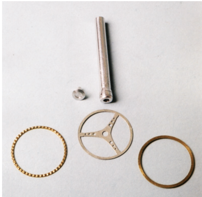
Figure 7.43: The steering column and Corvette steering wheel for DT 2 generally mimic the steering wheel from the pre-accident version of Spencer Murray's Dream Truck . The length of the column and its diameter, as well as the dimensions of the steering wheel and the spoke detail, were all taken from 1:1 scale parts.
