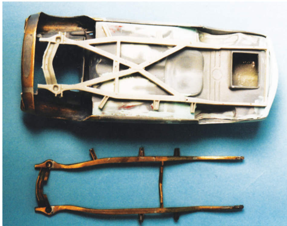
Figure 7.6: One way to create a body-on-frame model is to cut the frame away from a kit floorboard, and then cut the floorboard away from a frame on a duplicate part. Careful work will be required, and there will inevitably be work required to get everything to fit together. Here, an AMT '50 Ford frame has been cut in this manner, with work now going on to fit the floorboard to the body. The plastic frame can also be cast in brass for a more substantial element to the model.
