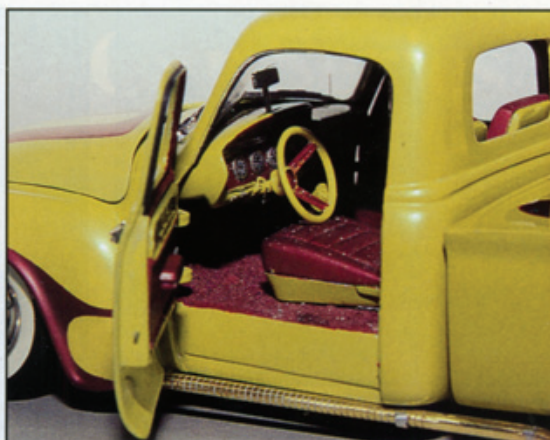
The interior components are painted to match the exterior. A low gloss clear has been applied over the 1962 Chevy bucket seats for a realistic vinyl look. The dash is poorly designed: The steering column is too low, dropping the small steering wheel almost to the seat. The gauge cluster needs to be raised to permit the steering column to be moved to a more realistic elevation.
