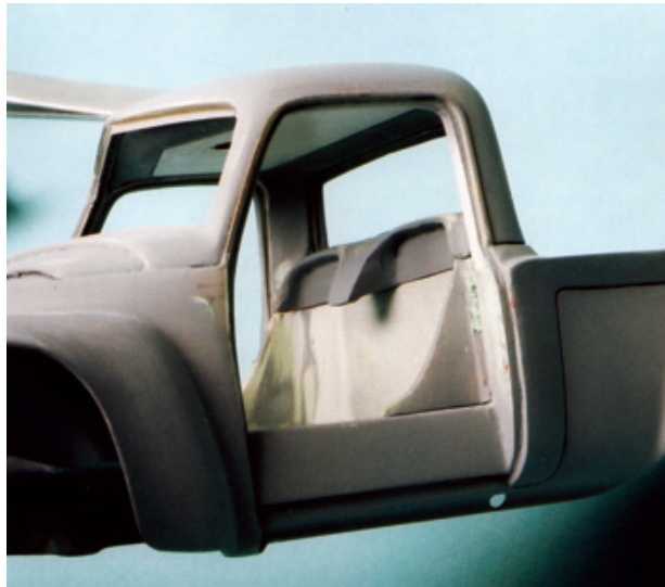
Figure 7.50: The seat surround, shown in its early stage, is placed inside the cab and beneath the headliner/rear window insert. Note how the shape of the upper seat receiver will sweep up and around and follow the side of the seat. Eliminating or minimizing the part-mating line between these two parts will be a challenge; either a piece of trim to cover the interface or a very tight line will be necessary. Again, prepare an assembly manual to govern construction; there is only one sequence that allows the interior of the DT 2 to go together.
