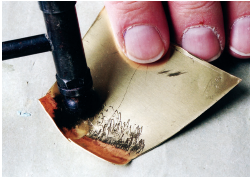
Figure 10.44: Now, let's start hammering. Determine the location of the “deepest” part of the curve, and start to lightly tap the back side of the sheet brass in the area. Don't assume that you can quickly shape the panel—dozens and dozens of light taps are needed. Vary the location of the taps and radiate the taps away from the sharpest part of the curve. In this photo, the location of the taps show up as shiny areas on the brass.
