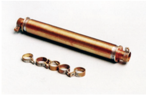
Figure 7.42: The tubular mufflers will mount inside the frame rails and will “hang” on the small machined/soldered brass “hangers.” Those clamps will be attached to photoetched hangars insulated by “rubber” straps “bonded” to a bracket that will be bolted to the frame. Of course, the diameters of the inlet and outside muffler clamps, as well as the hangers, match commercially-available brass tubing. Since DT 2 will be built as a “show truck,” all chassis-mounted exhaust parts will be nickel plated, and the lake pipes will be chrome plated.
