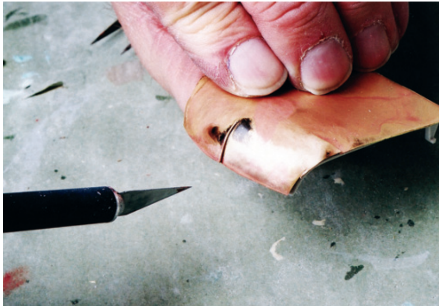
Figure 10.46: Relief cuts need to be made on both sides of the hood, as shown. The vertical line at the front of the hood is the cut made initially in the tape pattern—note how shaping the panel has closed the gap. The uneven bottom edge on the front of the hood is not problem—this is the natural result of the hammering process. We'll trim it later.
