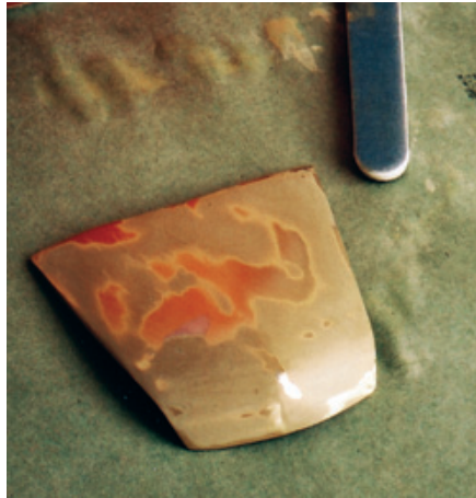
Figure 10.58: Lightly sand the hood once the Variprime has thoroughly cured (it sets up catalytically rather than “drying” in the traditional sense). Use a medium sanding stick and warm water. Check out the shiny areas which reveal high spots. Only by doing this kind of sanding will you ever get a perfect surface for painting. Gently tap down the peak of the high spot (this won’t dislodge the putty underneath), resand, and apply more Variprime. When cured, sand again.
