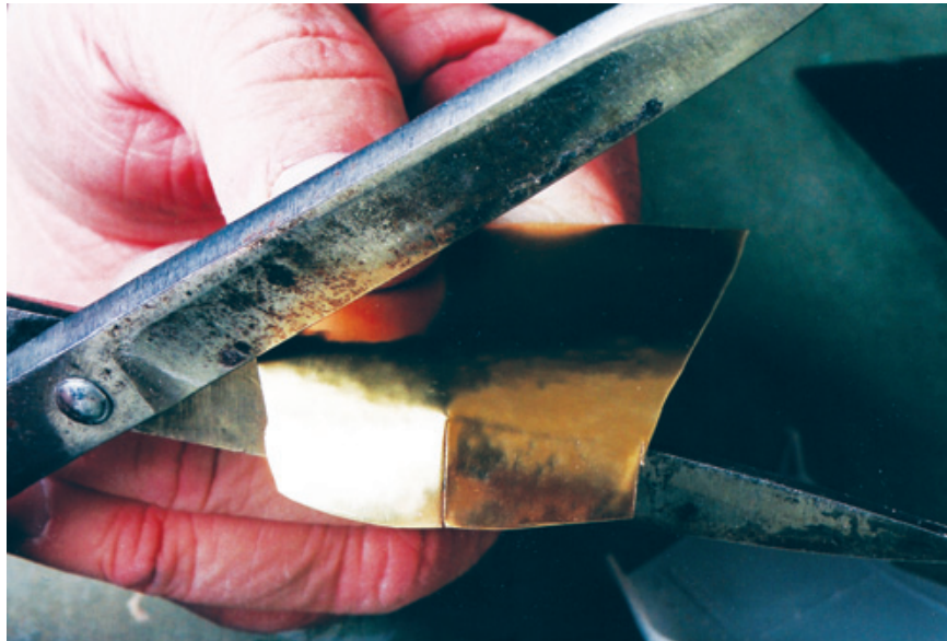
Figure 10.45: Note here how the leading edge of the hood has already started to curl. At this point, 40–50 hammer taps have occurred. You should make sure that both sides of the hood, measured by the centerline, are shaped concurrently to better insure uniformity. Remember that you are stretching the metal when you shape it with the hammer. Note how the center cut made earlier Figure 10.43 has begun to close up.
