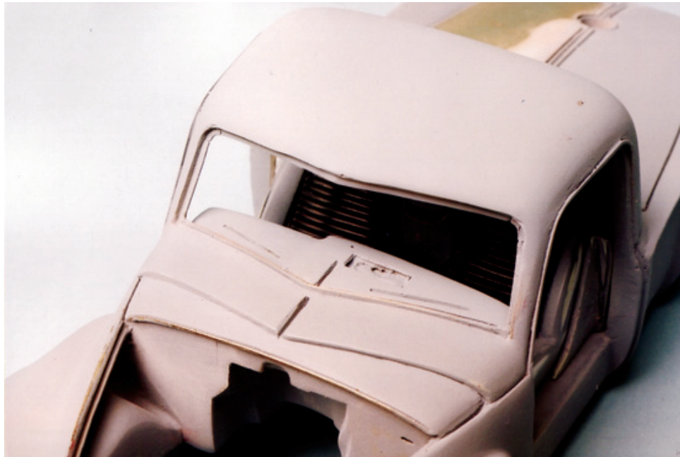
Figure 7.53: The first thing to do is to create a “ledge” against which the real glass, and the inside and outside trim, can be placed. The ledge here was created from “T”-shaped brass available from Special Shapes. Care must be taken to place this ledge, with respect to the windshield opening, so that inner and outer photoetched trim can fit without protruding beyond the dimensions of the surrounding body. See Figures 7.54 through 7.56.
