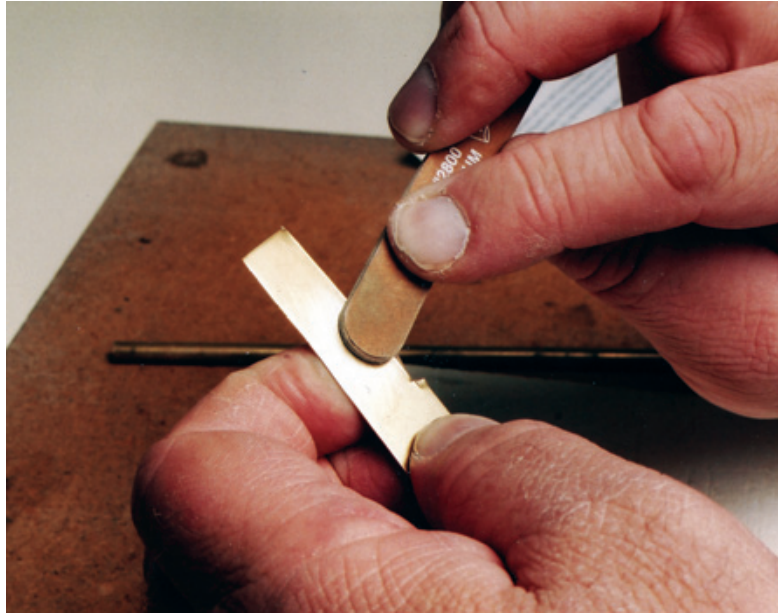
Figure 10.4: The first thing to understand about soldering is that you can "weld" parts together only if both surfaces are free of dirt, corrosion and other surface contaminants. Always lightly rough-up the surfaces. In this case, the flat surface is a piece of .025 K&S brass.
