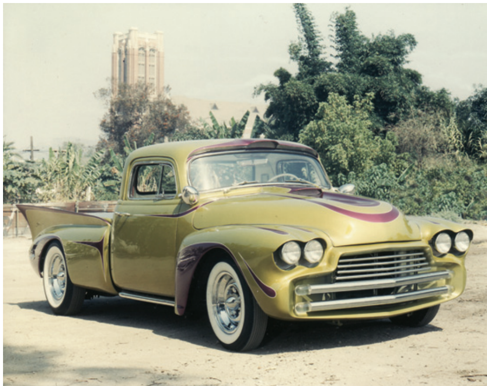
Figure 4.4: The last pre-accident version of the Dream Truck exhibited a number of obvious and subtle changes from the previous versions. For instance, the leading edge of the finned bed was straightened downward, the three Buick portholes-to-a-side were eliminated, and the paint scheme changed.
