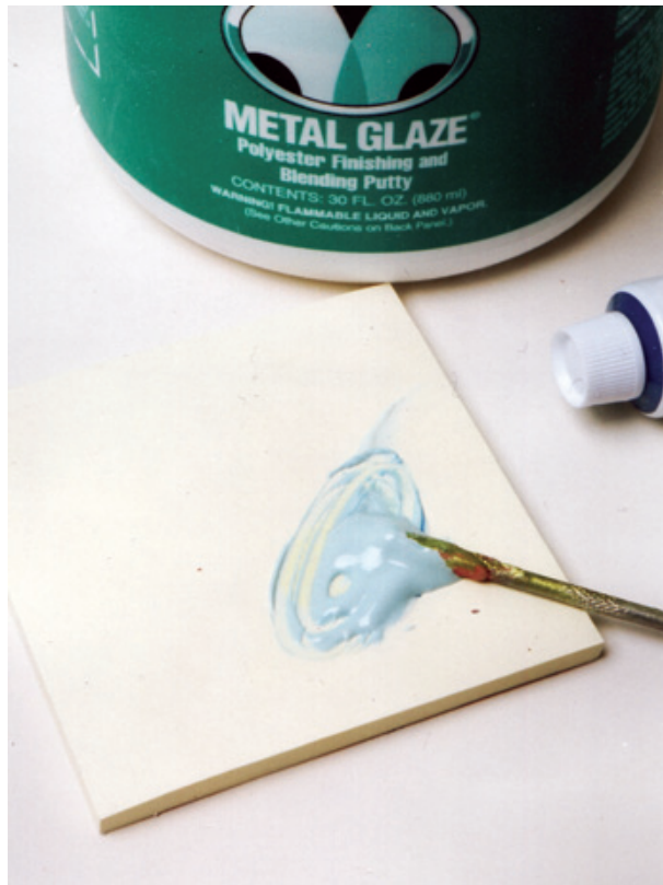
Figure 9.8: Mix the polyester putty carefully and completely. The more catalyst you use, the darker the mixed color becomes and the quicker it sets up. Experiment so that you create a mixture that cures in about three minutes.
