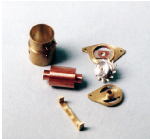
Figure 7.31: Similarly, the generator ( Dream Truck 2 is built to 1961 mechanical standards) is a multi-part assembly, and everything goes together easily. The armature was turned from copper to simulate the armature windings when it is seen through the small “windows” in the generator housing.
