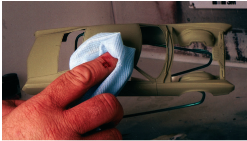
Figure 11.10: Lightly wipe down the model after first washing it again with liquid soap and water. Strict attention to cleanliness is essential to a show-winning finish.
