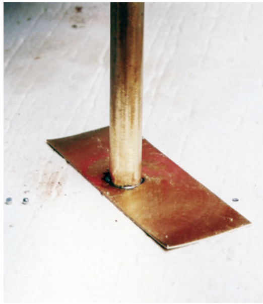
Figure 10.20: As the solder melts, it will naturally flow around the circumference of the joint and fill the gap. In fact, the solder “crawls” up the inside and the outside of the joint, thereby strengthening it.
