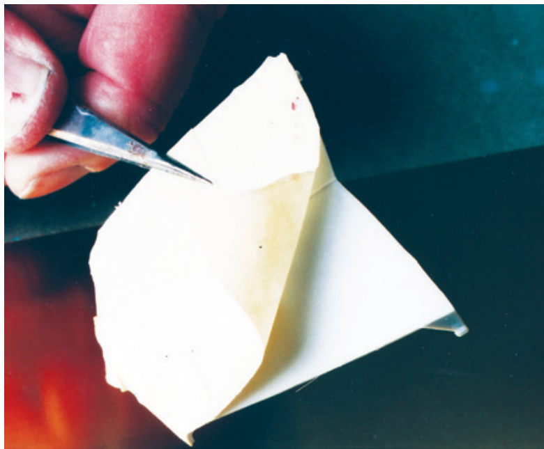
Figure 10.39: Carefully pull up the tape, being careful not to stretch the tape too much.
