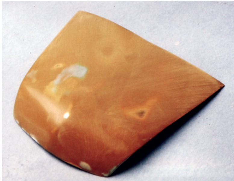
Figure 10.61: We're about done. More sanding revealed a slight low spot filled with a bit of catalyzed putty here. Use a medium sanding stick here and cross-sand the shape to show any slight surface irregularities.
