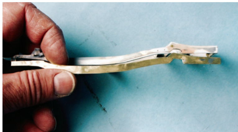
Figure 10.23: I traced one side of the plastic frame onto card stock, double-checked it for accuracy, and then traced around the card stock template onto a sheet of .025 brass. Because some material is inevitably lost when the frame rail sides are filed, it is important to start with frame rail material not less than .025 in thickness. Using a pair of carbon steel shears, cut out the pattern, then compare it to the plastic master frame; some correction was necessary.
