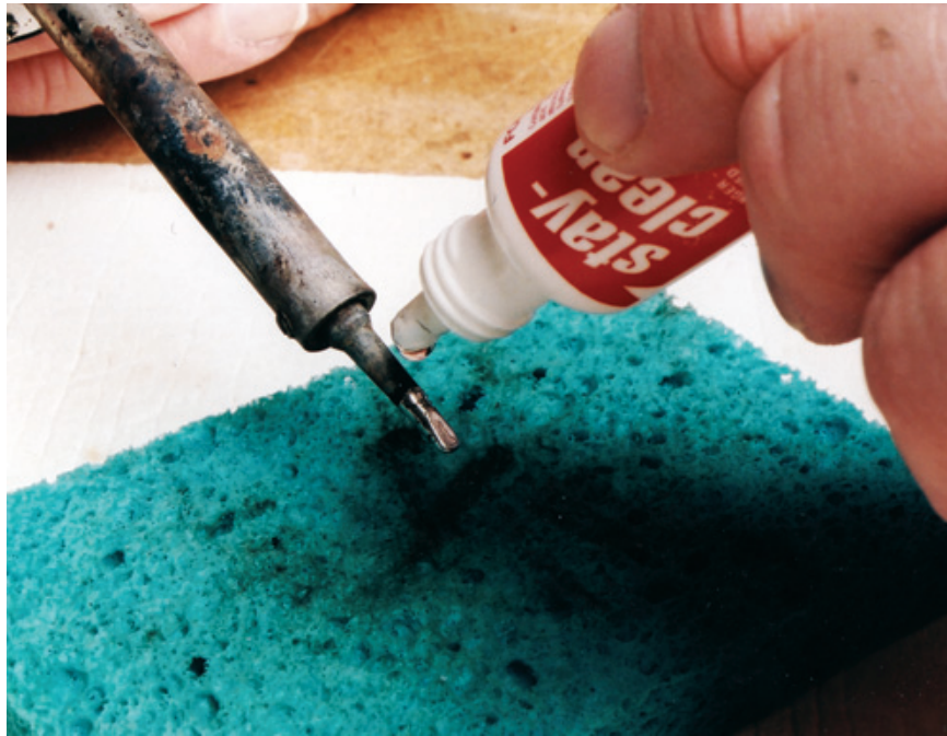
Figure 10.6: It is also important to keep the tip of your soldering iron clean. After each use, lightly wipe your hot iron across a wet sponge which will remove flux, excess solder and other contaminants. In this case, a small drop of liquid flux is being dropped onto the tip of the soldering iron as it is heating up. Remember, a soldering iron is hot, so be careful.
