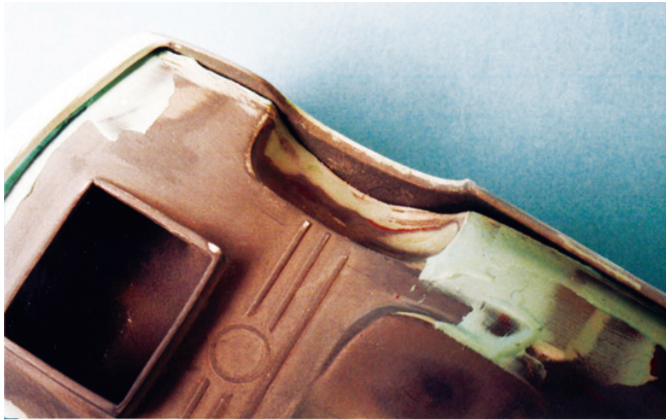
Figure 7.7: One task is to get the floorboard to mate up tightly against the body panel. Once everything fits, and the doors are cut out, and the floorboard can be correctly installed into the main body. Here, this process is in an early stage, with strip styrene being applied around the rear wheelhouses so that there is almost no gap between the body and floorboard. Be careful to correctly locate the floorboard, since it will also locate the frame, and you want to be certain the axles are correctly placed on the model. Take your time here.
