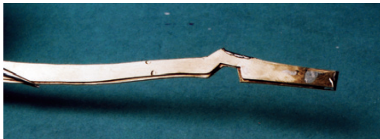
Figure 10.26: Choosing the closest matching dimensions, the soldering iron was used to solder the rails together by “spot soldering” the two parts in just a few key points. At this point, the larger (second) of the two frame rails was filed to match the smaller (first) frame rail. When both parts matched, the torch was used to heat up the several soldering spots and the two rails were pulled apart, and the solder points were carefully filed away. These frame rails could have been photoetched, too.
