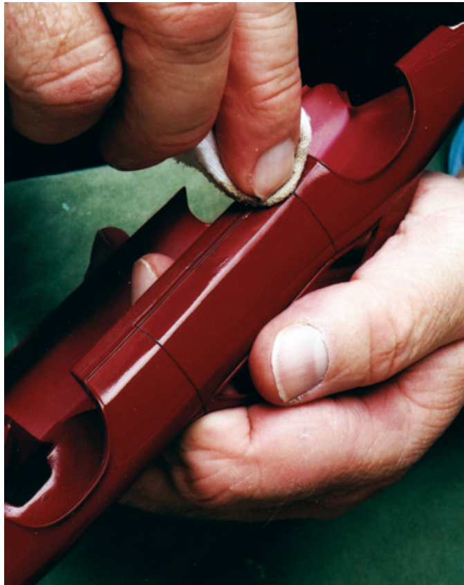
Figure 11.23: In small areas adjacent to sharp panel lines, approach the area from opposite the crease, never over the top of the line. Gently rub along the length of the inside of the crease line. Think about what you're doing, and remember that polishing removes a bit of paint in the process.
