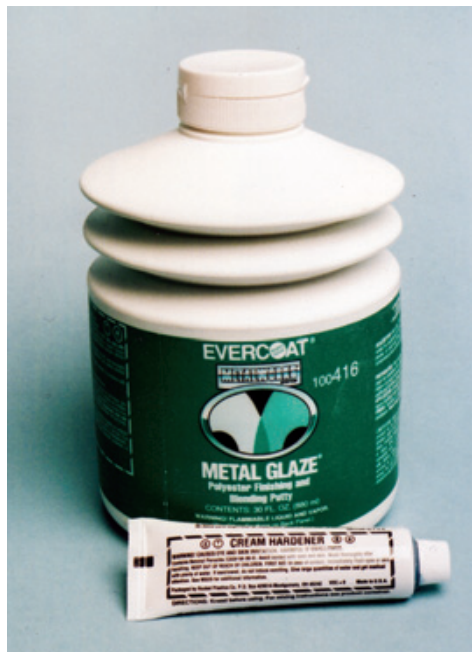
Figure 9.1: The polyester two-part putty marketed by Evercoat is the best catalyzed putty to use. Formulated for use with automotive paint, this is an excellent product that requires mixing the putty with a catalyst. Choose the “Metal Glaze” version from the Evercoat line; it is finely-grained and feather-edges beautifully. Remember to keep the lid on tightly; otherwise, you’ll have a solid two-pound paperweight! Other brands are also available.
